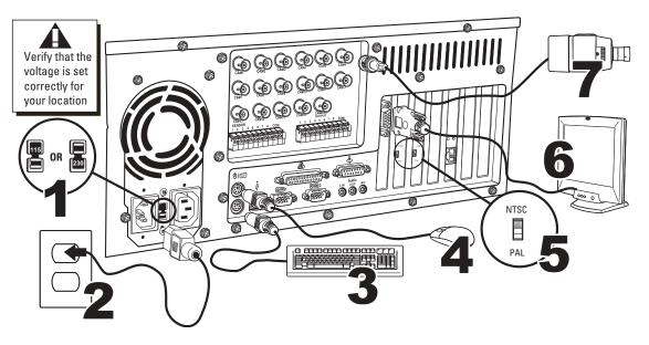
Figure 3. Basic Equipment Installation
